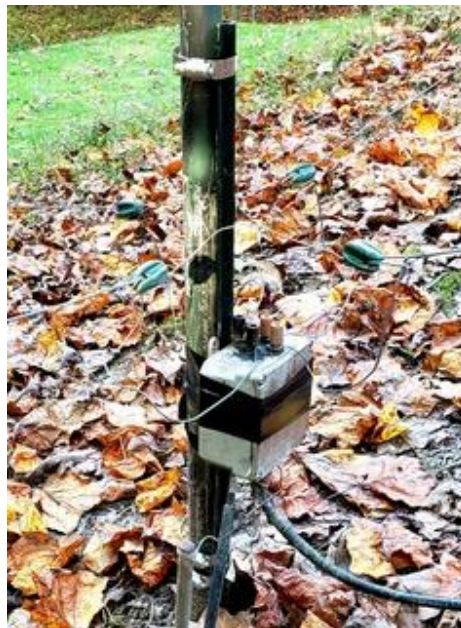
Fig. 4 A large U-post supports the 25' fiberglass Center support and control box for the K9AY loop at N4GG. The control box is taped to the U-post—low tech but it works.
