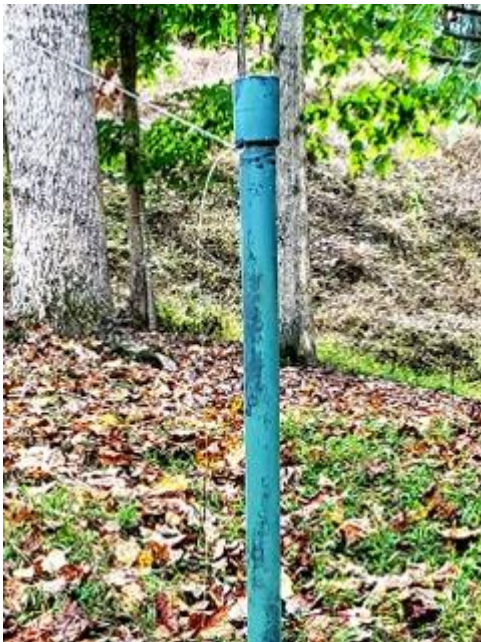
Fig. 3c K9AY Loop Tie-point
