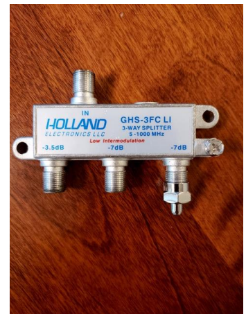
Figure 5 Unused Port Terminated
