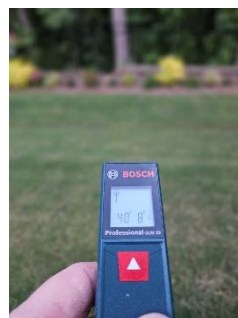
Figure 2. A Bosch GLM-20 measuring the distance to a tree.
