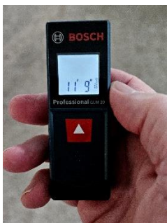
Figure 1. A Bosch GLM-20 measuring distance to an interior wall. Maximum capability is 65 feet.
