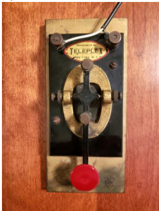
Figure 1. My first and only straight key. Used for code practice in 1960 and my Novice days (1961). Call sign WV2QPW. It is still used occasionally on the air. The heavy steel base was a gift from Frank Leonard, W2NPT, in early 1960.
