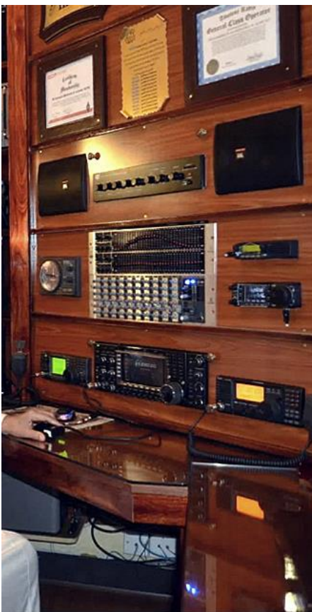
Figure 2. A station where everything is built-in. There is no room for the operator's arms. This station would not be fun to operate.
