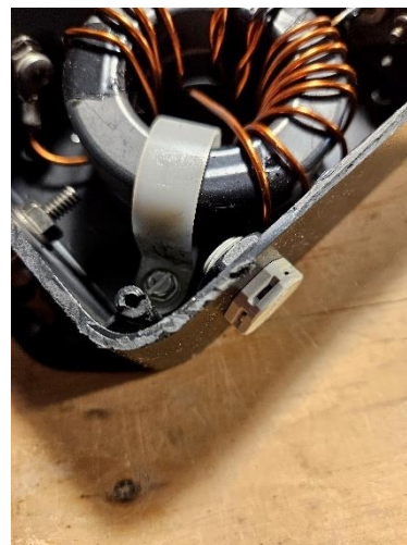
Figure 2 Inside view of the "1 KW ICAS" rated EFHW matching box.
