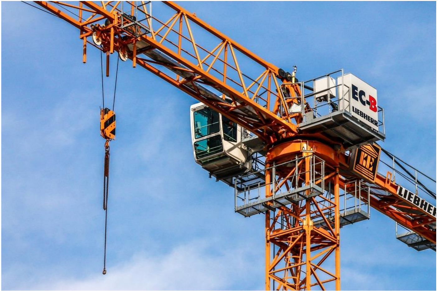
Figure 2. A close-up of the rotating shack. It has a nice stiff 480VAC 3 phase power system.
